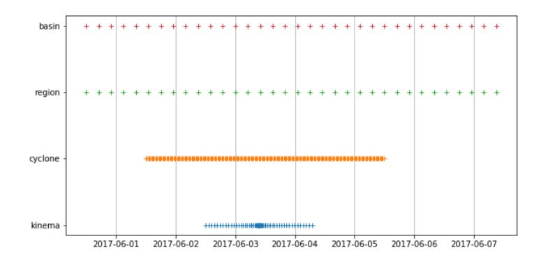
Example of independent time-stepping for each overlay, including individual start/stop and non-regular timestep intervals.
