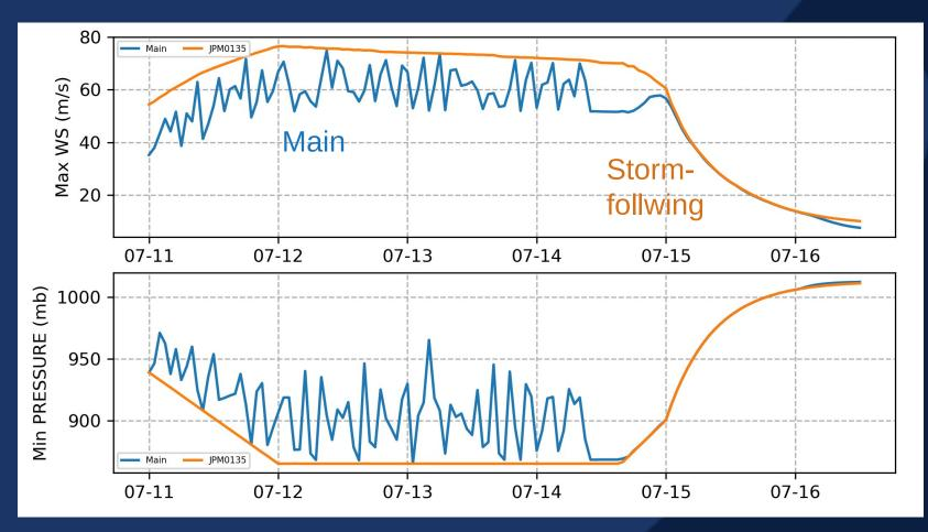
Time evolution of maximum wind speed (top) and minimum surface pressure (bottom) by sub-grid/overlay for JPM 135, 1-hour input timestep
