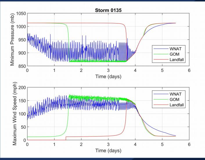
Time evolution of min pressure (top) and max wind speed (bottom) by sub-grid/overlay (including a 3<sup>rd</sup> Gulf of Mexico domain (GOM, green)) for JPM 135 as NWS12 files with 5 minute input timestep
