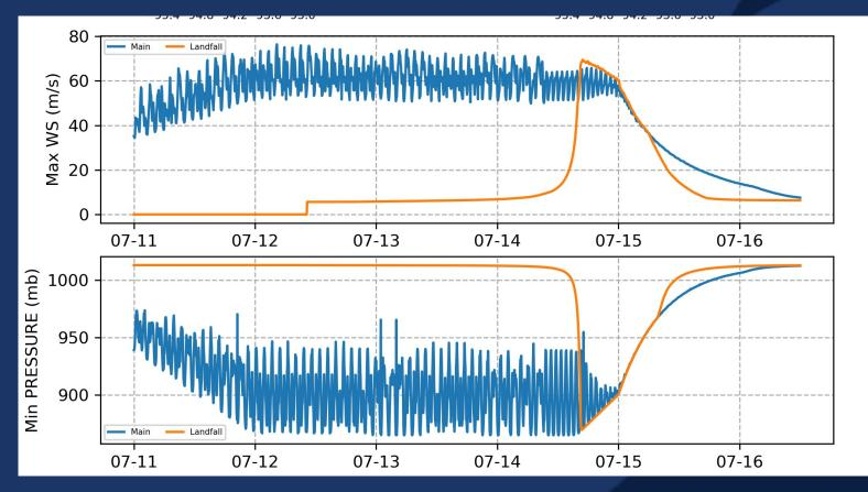
Time evolution of max wind speed (top) and min pressure (bottom) by sub-grid/overlay for JPM 135 as NWS12 files with 5 minute input timestep
