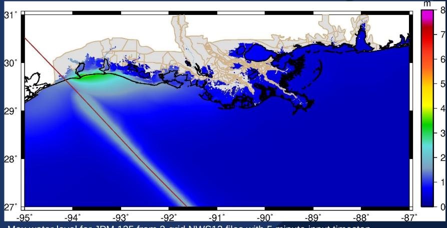
Max water level for JPM 135 from 3-grid NWS12 files with 5 minute input timestep
