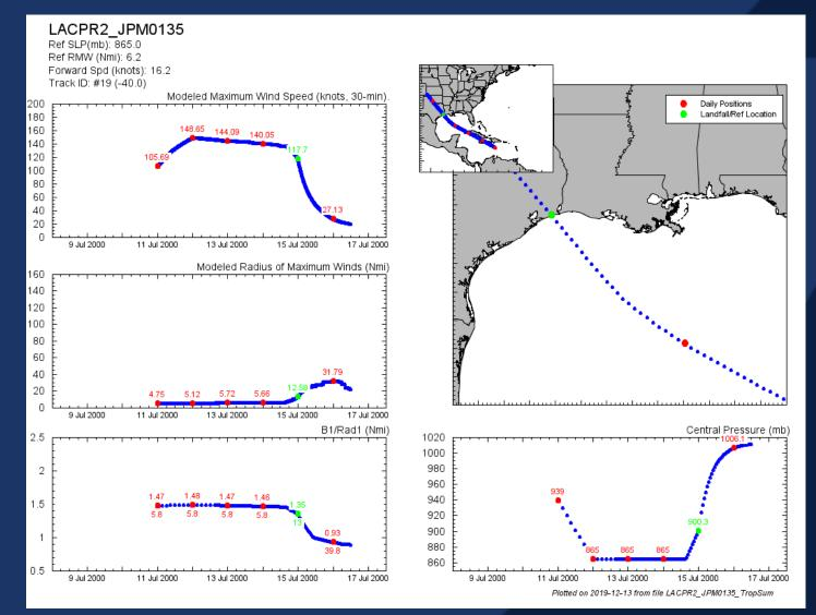
Diagnostic information for synthetic JPM storm 135, demonstrating relatively tight, intense, and fast moving storm.
