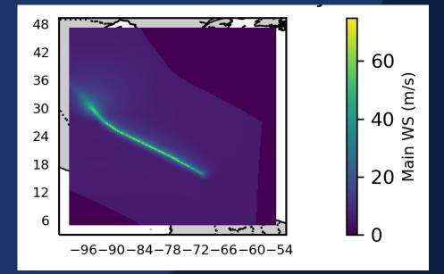
Max wind speed on "Main" mesh-wide input grid
