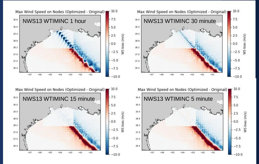
Difference between the NWS 12 (5 min input timestep) and 13 (1 hour input timestep) max wind speed representations interpolated by ADCIRC on to a mesh for various WTIMINC in the NWS-13 cases.
