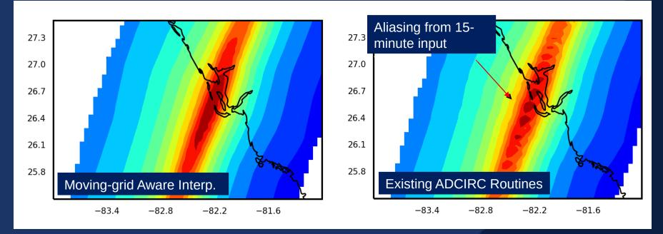
Max wind speed plots showing the impact of intelligent moving-grid aware interpolation routines (left) compared to a fixed 15-minute timestep (right) from fast moving Hurricane Charley (2004) as it makes landfall in Florida.
