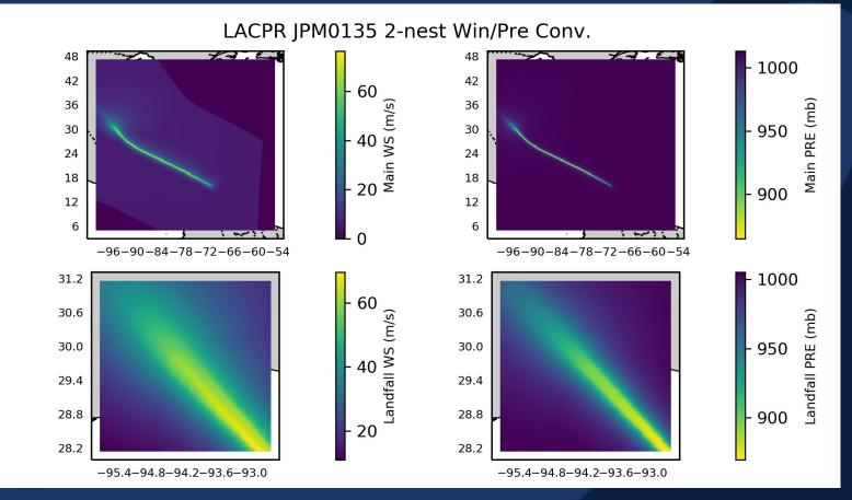
NWS 12 max wind speed (left) and min pressure (right) inputs on basin-wide (top) and landfall (bottom), 5 minute input timestep
