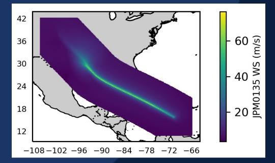
Max wind speed for the storm-following input grid
