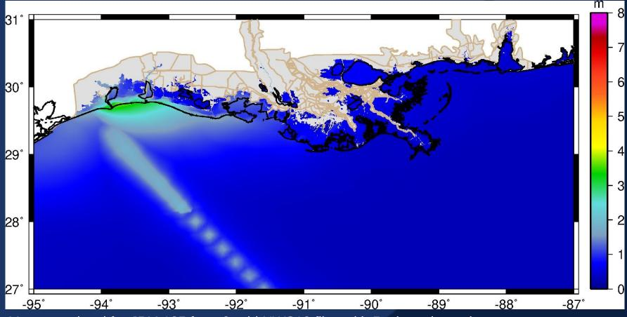
Max water level for JPM 135 from 2-grid NWS12 files with 5 minute input timestep
